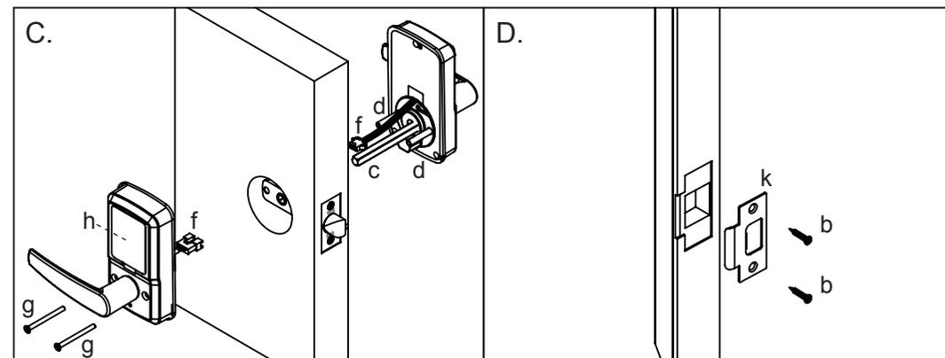
Insert the square spindle (c) through the door and latch (a). Connect the wires (f) x 2. Connect the two plates and tighten screws (g) x 2 into pipes (d) x 2. Remove battery cover (h) and install 4 AA batteries.
