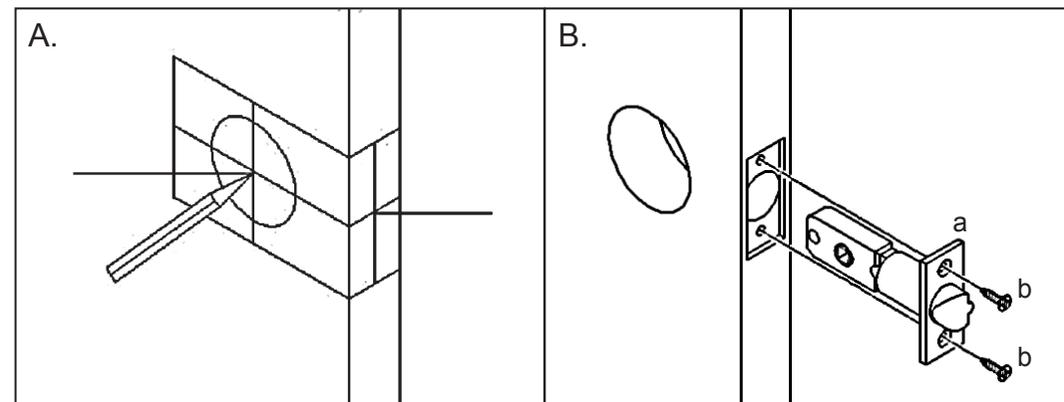
If the door is not bored, use the attached template and follow instructions on it. If the door is bored, skip Step A and proceed to Step B.
